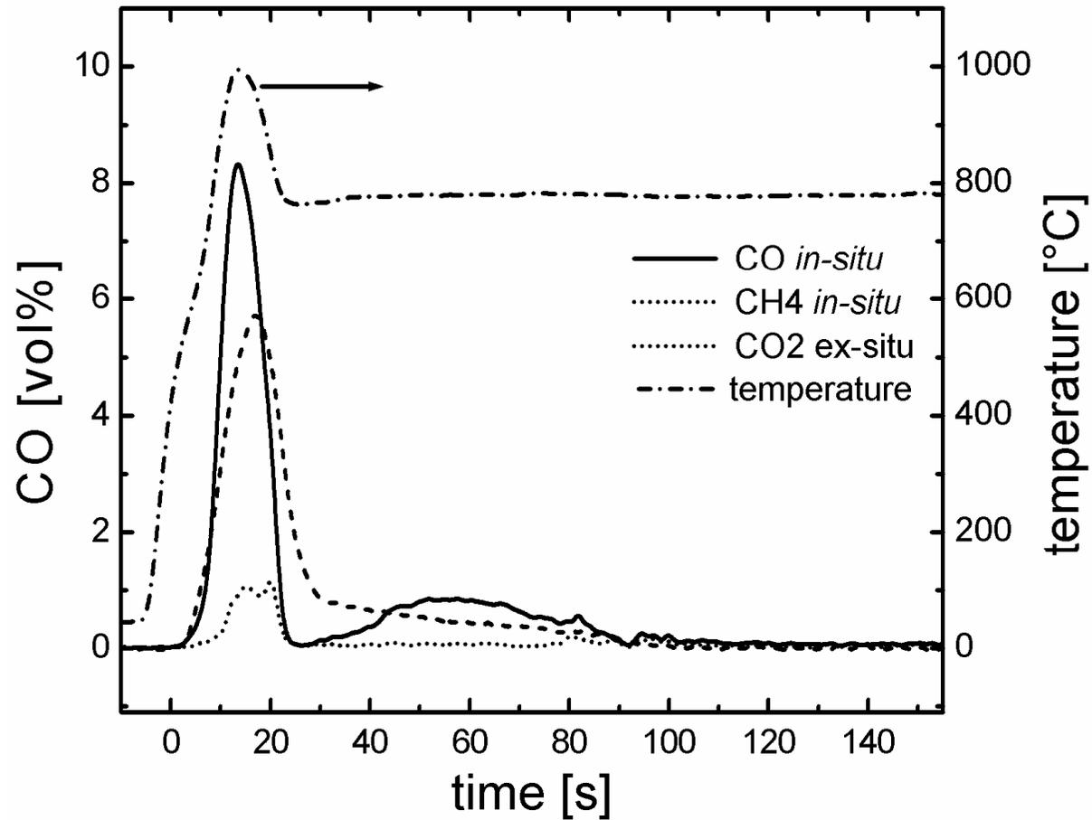
800°C, 15kPa O<sub>2</sub>, 10 mm distance, 0.5 g beech wood, Ø 4mm
