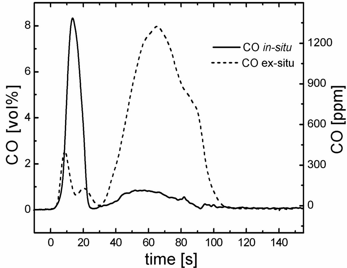
800°C, 15kPa O<sub>2</sub>, 10 mm distance, 0.5 g beech wood, Ø 4mm
