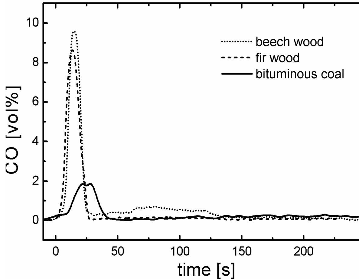
800°C, 10kPa O<sub>2</sub>, 10 mm distance, sample mass 0.5 g wood, 1.0 g coal
